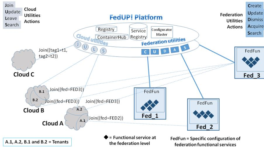
Fig. 1. A conceptual overview of the proposed solution
