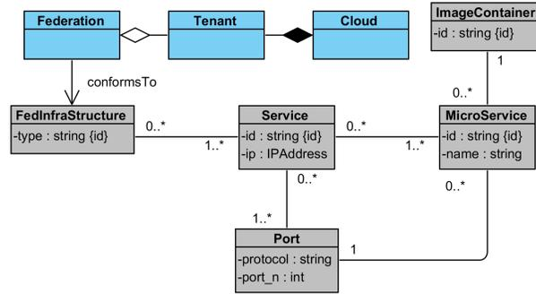
**Fig. 3.** The metamodel for the federation infrastructure
