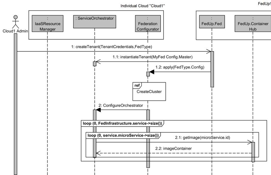
**Fig. 4.** The sequence diagram for creating a federation
