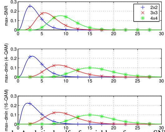
Fig. 1: Analytical pdf of variable  $z$  for  $\max\text{-SNR}$ , 4-QAM and 16-QAM  $\max\text{-}d_{\min}$  precoders.
