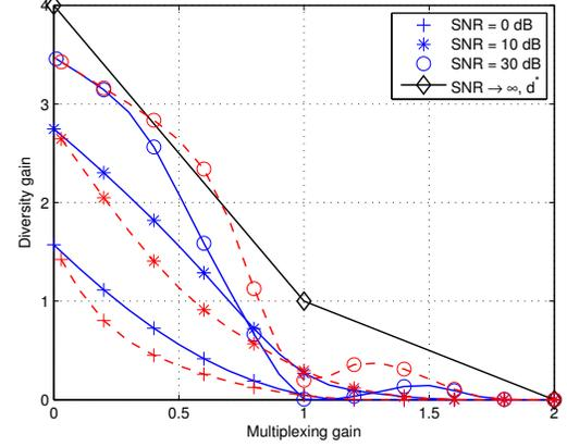
Fig. 3: Finite-SNR DMT curves for the max- $d_{\min}$  precoder and  $2 \times 2$  MIMO system. The optimal solution for 4-QAM is in blue solid line, and the optimal solution for 16-QAM is in red dash line
