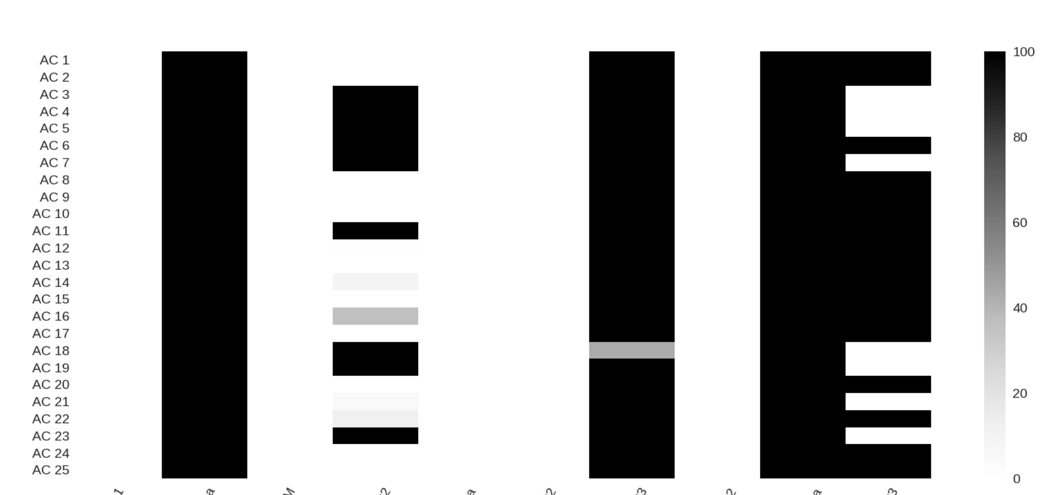
Figure 2: Bolasso selection for L features of 25 similar A/C. Each row corresponds to a different A/C and each column to a different possible feature. The cells color indicates the selection frequency over 128 Lasso s solved. Training was performed using 10 471 302 observations in total.
