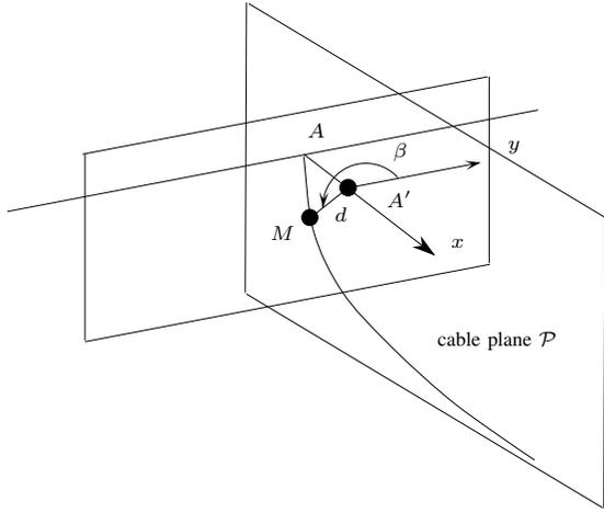
Fig. 5. A new sensor arrangement for measuring the  $\theta_V, \theta_H$  angles. A range meter is mounted on a rotary head located at  $A'$  rotating around the  $x$  axis. The range meter is rotated until it detects the cable and the system provides the distance  $d$  between  $A'$  and the cable and the rotation angle  $\beta$
