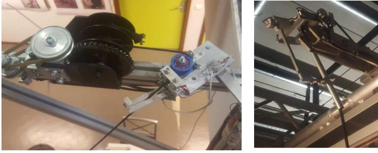
**Fig. 2** On the left the rotation guide of MARIONET-Assist which allows for the measurement of  $\theta_V$ . On the right the system used on MARIONET-VR for the measurement of both  $\theta_V$  and  $\theta_H$
