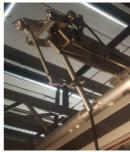
Fig. 2 On the left the rotation guide of MARIONET-Assist which allows for the measurement of  $\theta_V$ . On the right the system used on MARIONET-VR for the measurement of both  $\theta_V$  and  $\theta_H$
