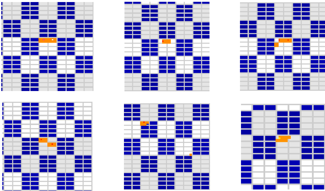
Figure 5: Different blocking pixels (in red and yellow) configurations and resulting blocked warps (in orange)
