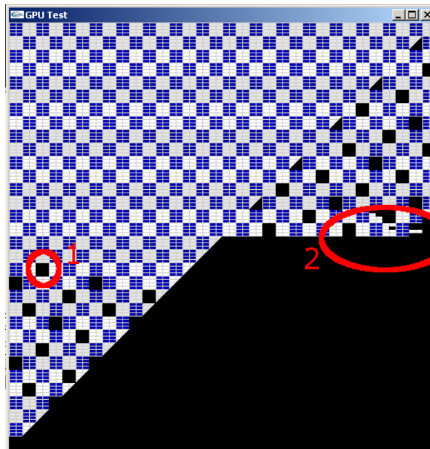
Figure 2: A tile containing a very slow fragment (1) makes all next tiles scheduled on the same TP to wait. Others TPs continue their processing until their fragments FIFO is empty (2).
