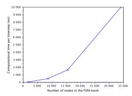
Figure 8. Relative error (left) and computation time (right) of Diamond robot simulation when varying the refinement of the mesh. The relative error is computed for the end-effector position when actuating three of the four cables.
