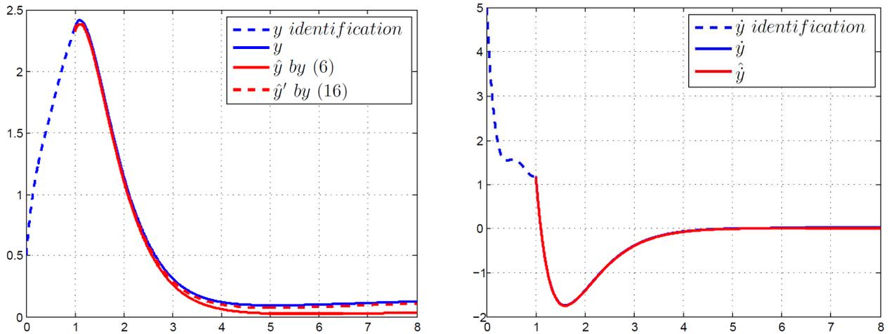
Fig. 3. Position and velocity for robust controller
