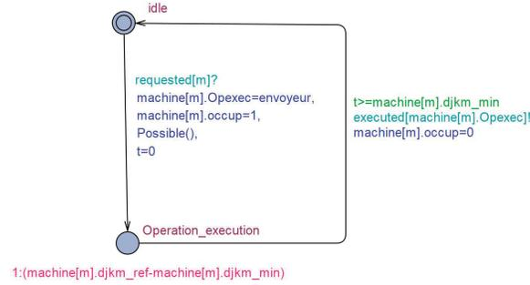
**Fig. 3** Model pattern  $\beta^m$  for the machine  $m$
