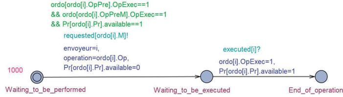
**Fig. 2** Instantiation of an operation pattern using UppAal
