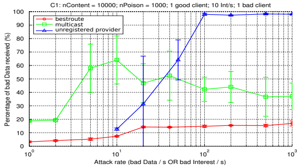
Figure 2. Attack rate effect on the legitimate client
