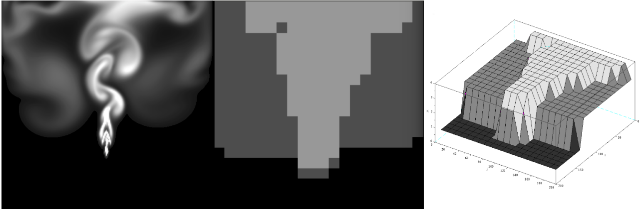
Figure 1: Fluid simulation snapshot (left), corresponding monitored state grid (center), generated computation volume (right)
