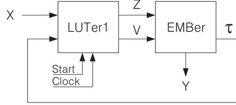
**Fig. 4.** Structural diagram of Moore FSM  $U_3$
