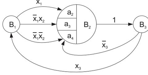
**Fig. 3.** Class transition graph for Moore FSM  $S_1$ **Table 1.** Structure table of Moore FSM  $S_1$
