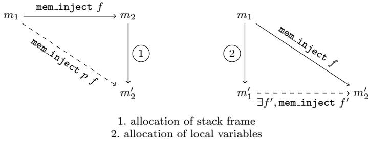
Fig. 23: Structure of `match_callstack_alloc_variables`'s proof in CompCert
