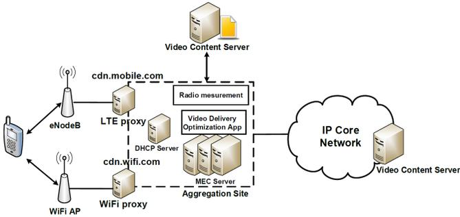
Fig. 1: Our MEC-assisted mobile adaptive HTTP streaming architecture.
