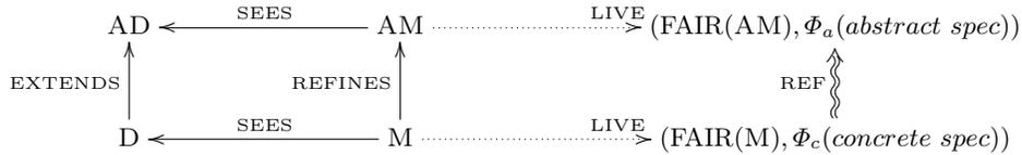
Fig. 2. Summary of the integrated formal methods refinement methodology
