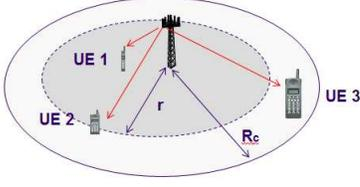
Figure 1. Cell of radius  $R_c$ . SIC: user UE 2, located at  $r$ , is able to decode the power dedicated to any user UE 3, located at a distance greater than  $r$  (white area). The power dedicated to any user UE 1, located at a distance lower than  $r$  (grey area), cannot be decoded by user UE 2.
