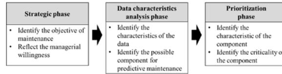
Fig. 2. Decision-making process for applying predictive maintenance.
