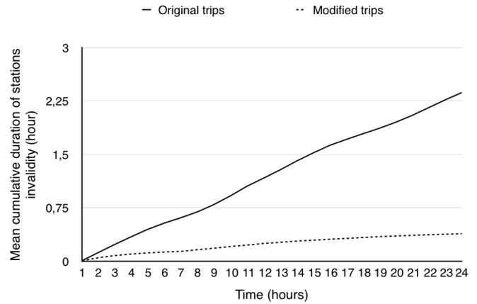
Fig. 10. Mean cumulative duration of stations invalidity
