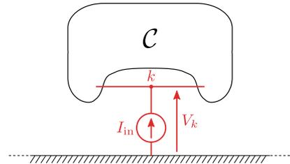
Fig. 7. Partial transfer function at node  $k$
