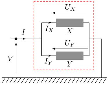
Fig. 10. Composition of one-port circuits in parallel
