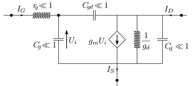
Fig. 16. Intrinsic model of a linearized transistor
