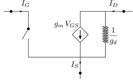
Fig. 6. Model for the linearized controlled current source.
