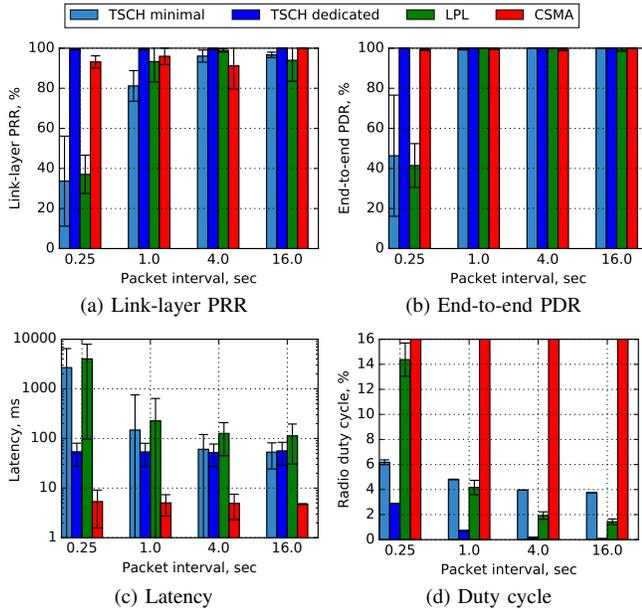
Figure 4. **Comparison of TSCH with Low-Power Listening (LPL) and CSMA.** For TSCH, the 6TiSCH minimal schedule and a collision-free schedule are compared. Note the log y-scale used for latency. Note that the duty radio cycle for CSMA is 100%, not fully shown in the graph.
