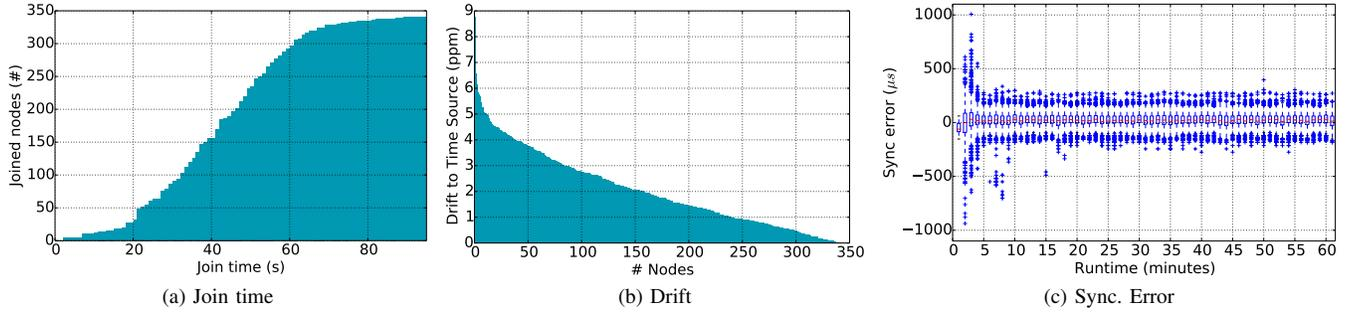
Figure 3. **Time synchronization experiment, 340 nodes.** (a) Shows the number of joined nodes at any given time after bootstrap. (b) Shows the distribution of the nodes’ drift to their time source. (c) Shows how synchronization errors evolve with time. The duty cycle converges to 0.3%.
