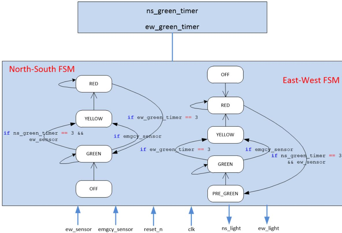
Fig. 12: Traffic Intersection Controller Module
