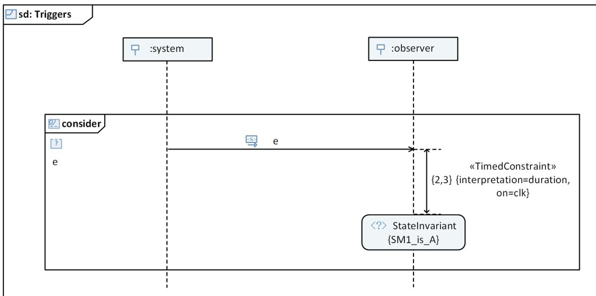
Fig. 9: e triggers A after [2,3] on clk
