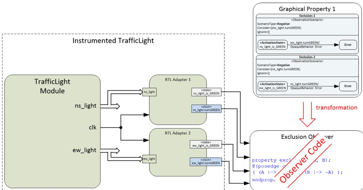
Fig. 17: Integration of Observer in the Verification Environment
