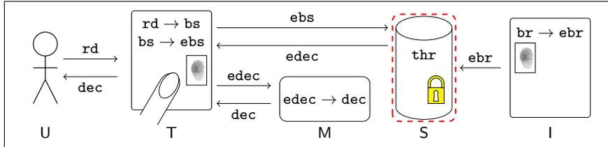
Fig. 4. Comparison over encrypted data with homomorphic encryption
