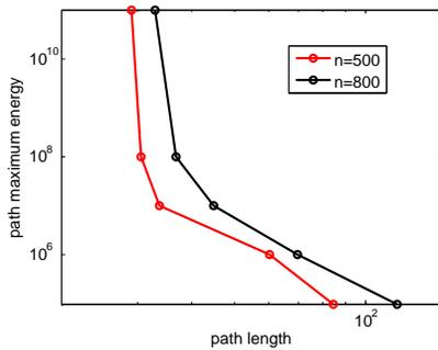
Figure 9: Path maximum energy versus hops  $d_m = 3.3, d_r = 2.3$
