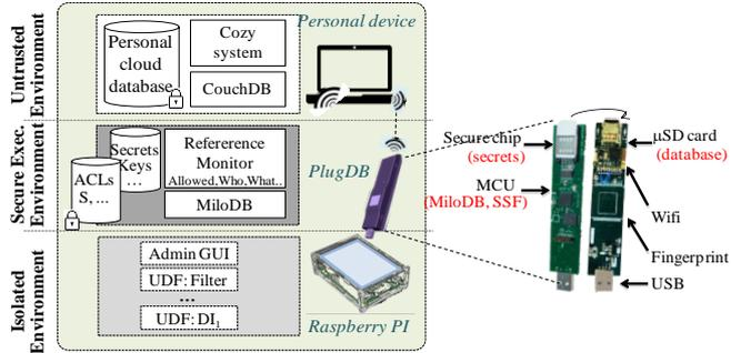
Fig. 2. Experiment platform: software and hardware (right).
