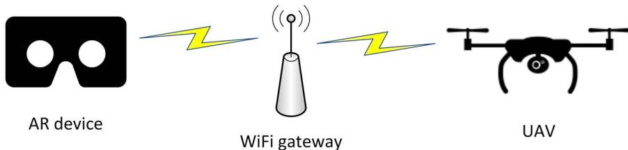
**Fig. 1.** Model of network for interaction between the AR device and UAV.
