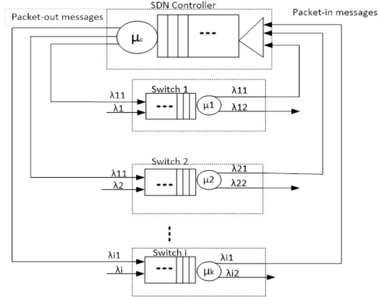
**Fig. 8.** OpenFlow-based SDN queuing model
