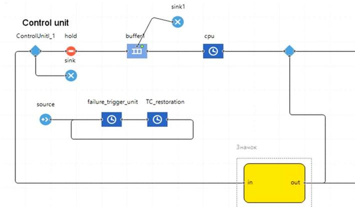
Fig. 5. SDN controller conceptual model in AnyLogic 7.3.6
