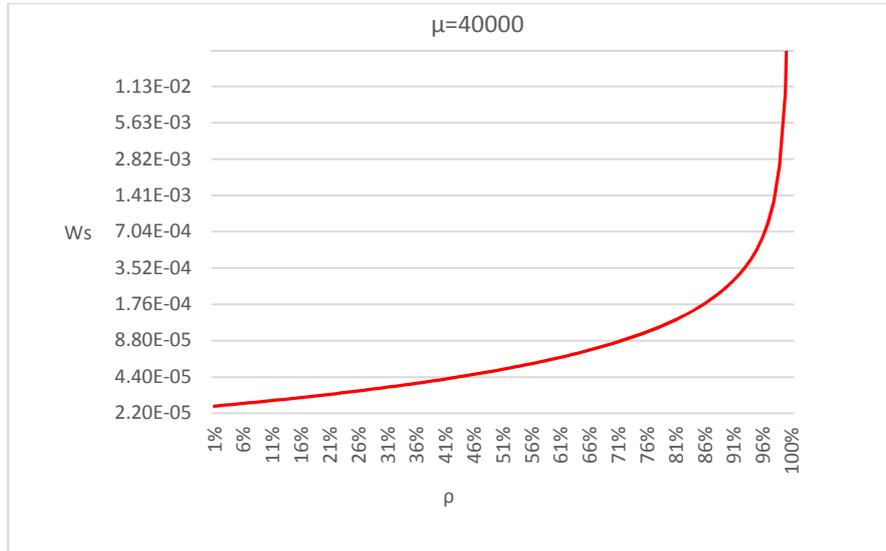
**Fig. 10.** Average packet processing time of Switch
