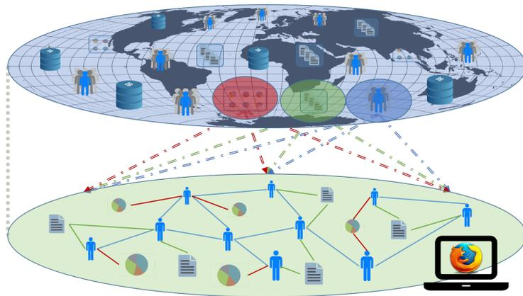
**Fig. 1:** Publish-subscribe mechanism used by a client to constantly synchronize a sub-sample of a *global database* to constitute what we term the *local sphere*. Note that the local sphere is a superset of the user's data - it may contain items a user is not actually requesting, but might be significant for computing relevant recommendations.
