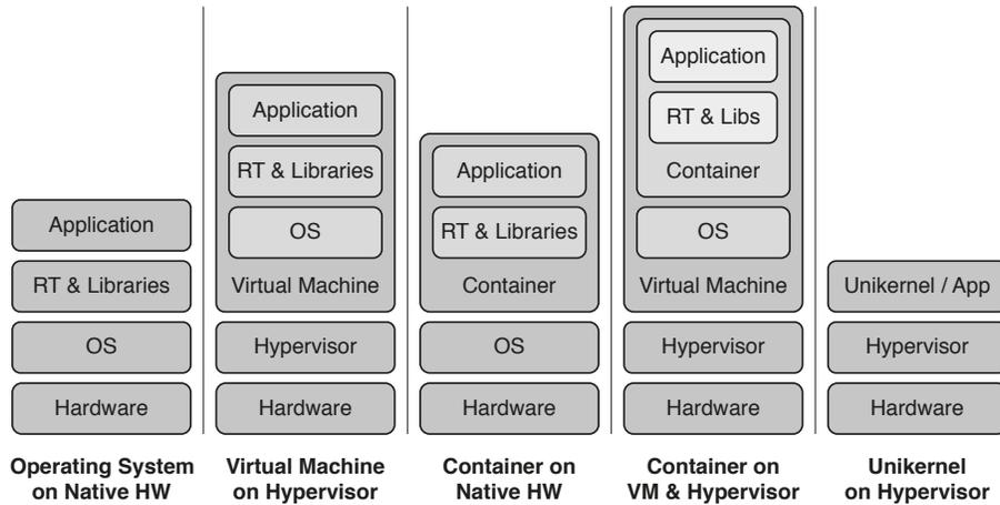
**Fig. 2.** Illustrated comparison of the software stack complexity of various deployment strategies, including native setups, virtual machines, containers, containers within virtual machines and unikernels.
