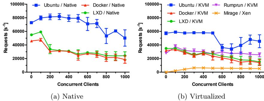
**Fig. 4.** Throughput of *Nginx* (1.8.0) was evaluated on native hardware (a) and in virtualized environments (b). For MirageOS, the *conduit server* was used. Throughput was measured using *weighthttp* and the modified *abc wrapper* utility.
