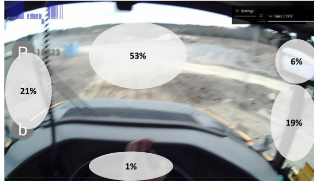
Fig. 6. Level of attention in different areas for articulated dump truck.
