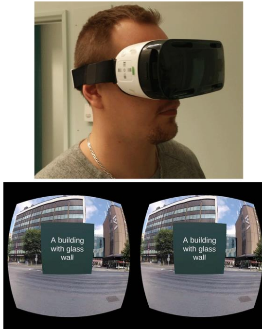
Fig. 2. Top: Amaze360 physical setup. Bottom: Amaze360 application view. The video is shown as a stereoscopic presentation. Activated hotspot is shown at the center of screen.
