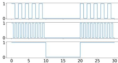
Figure 4. On the bottom, the red channel input with the regular  $f_{csk}$  CSK modulation. Above, the CSK modulation is combined with a  $f_{pwm}$  PWM and  $f_{pwm}/2$  PWM so that dark and light stripes will appear within the CSK symbol period.
