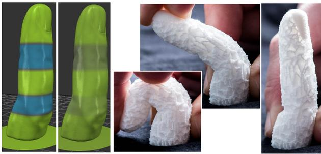
Figure 20: The articulations of this finger prosthetic are obtained by spatially varying density and anisotropy. The design is very robust and easy to print: it uses a rubber-like filament (*Cheetah* by *NinjaTek*) printed on a standard FFF printer (Prusa3).
