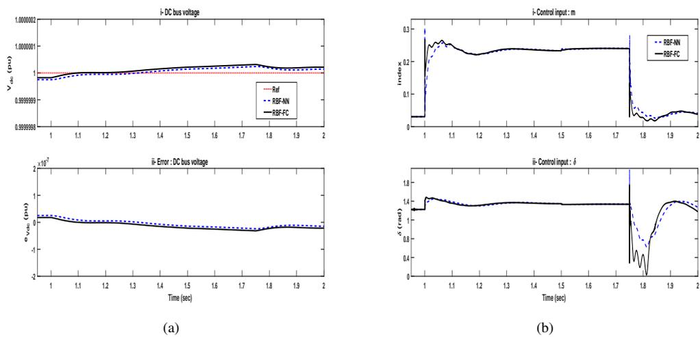
**Figure 5.** Control response to step changes in real and reactive powers of the transmission line under online variation of  $R_s$  (up to +40%) and online variation of  $X_s$  (up to +20%). (a) DC bus voltage of SSSC. (b) Control input of SSSC
