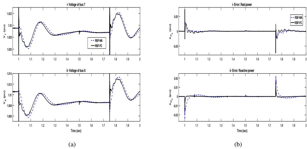
**Figure 4.** Control response to step changes in real and reactive powers of the transmission line under online variation of  $R_s$  (up to +40%) and online variation of  $X_s$  (up to +20%). (a) Voltage of bus 7 and 8. (b) Error on real power and reactive power
