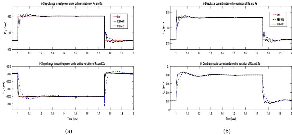
**Figure 3.** Control response to step changes in real and reactive powers of the transmission line under online variation of  $R_s$  (up to +40%) and online variation of  $X_s$  (up to +20%). (a) Active and reactive power in the transmission line. (b) DQ currents
