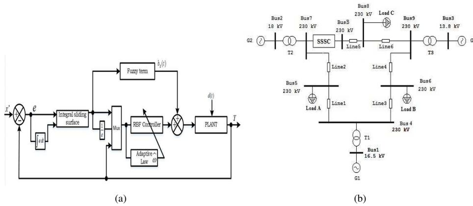
**Figure 2.** (a) Detailed block-diagram of the RBF-Neuro-Fuzzy controller. (b) IEEE 9 bus test system with SSSC device
