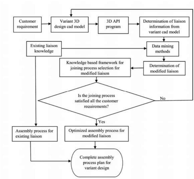
**Fig. 5.** A framework for variant design application
