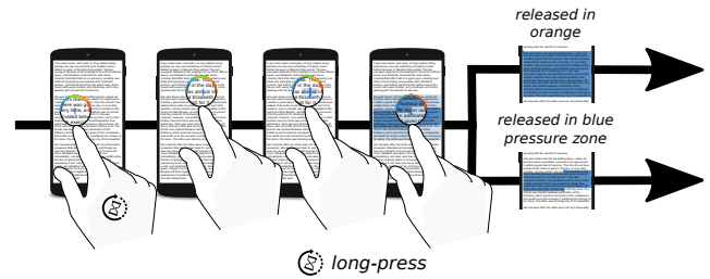
Figure 2: Example of text selection using FORCESELECT. The user performs a long-press that displays the callout magnifier. Keeping the force in the character level, the user adjusts its position by moving her finger. She then presses harder to start the manipulation of the second cursor. If she releases her finger while the force is at the sentence level of the “mode gauge”, she will select the whole paragraph. If she releases her finger while the force is at the character level, she will only select what is between the two cursors.
