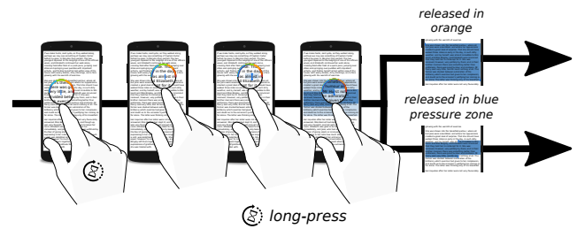
Figure 2: Example of text selection using FORCESELECT. The user performs a long-press that displays the callout magnifier. Keeping the force in the character level, the user adjusts its position by moving her finger. She then presses harder to start the manipulation of the second cursor. If she releases her finger while the force is at the sentence level of the “mode gauge”, she will select the whole paragraph. If she releases her finger while the force is at the character level, she will only select what is between the two cursors.
