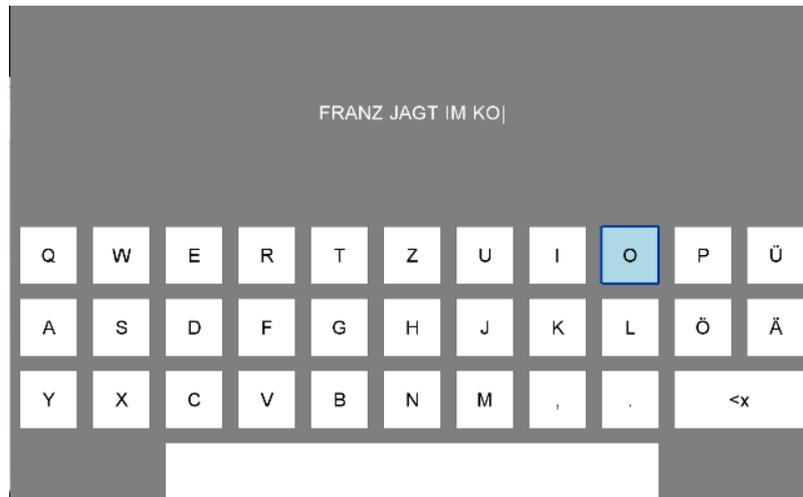
**Fig. 1.** Screenshot of the implemented on-screen keyboard. Gaze highlighted keys in light blue while a combination of pupil deviation criteria and fixation duration selected (highlighted by a dark blue frame).
