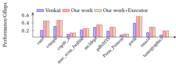
Figure 16. Performance of the CSR SpMV on CPU
