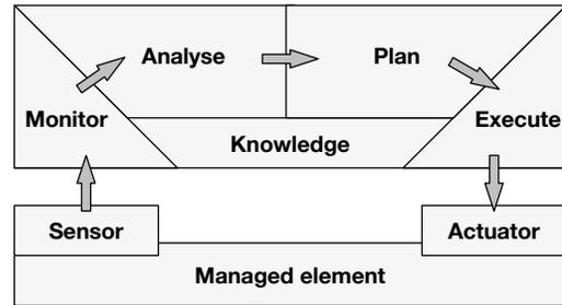
Figure 2: Overview of the MAPE-K loop process
