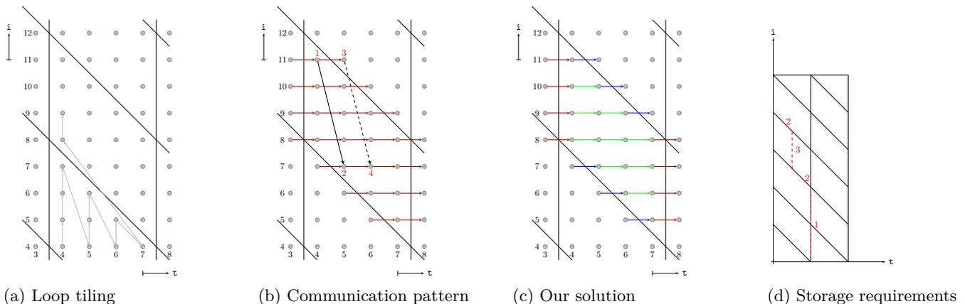
Figure 3: Impact of loop tiling on communication pattern
