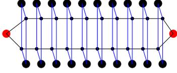
Fig. 3: A routing game made of one central (horizontal) flow with two possible routes (up or down) against  $n-1$  transversal (vertical) flows, each with two routes (left or right). The routes of the central flow share two hops with each transversal flow, but the routes of transversal flows do not intersect each other.
