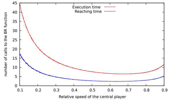
Fig. 5: Mean execution time and reaching time of Algorithm 4 over 10,000 random samples of the routing game displayed in Figure 3, when the relative speed of the central player ( $\frac{\lambda_0}{\lambda_0 + \lambda_1}$ ) ranges from 0.1 to 0.9.
