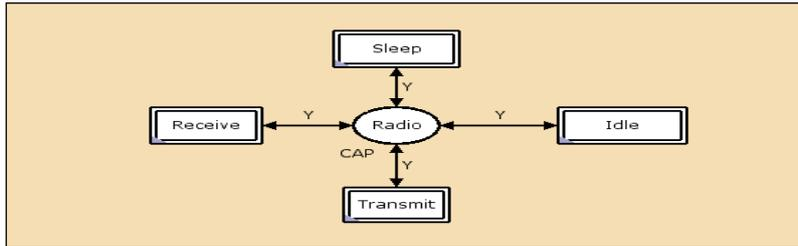
Fig. 1. The CP-net modeling the behavior of Radio component
