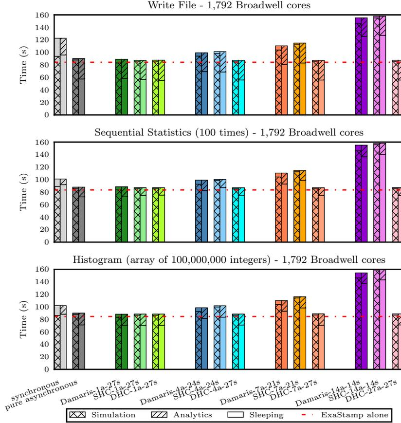
**Fig. 3.** Comparison of the different strategies on 1,792 Broadwell cores (64 MPI processes) for three analytics quicker than the simulation timestep: file writing (a), sequential statistics performed 100 times (b) and histogram with an array of 100,000,000 integers for the MPI collective communication (c).
