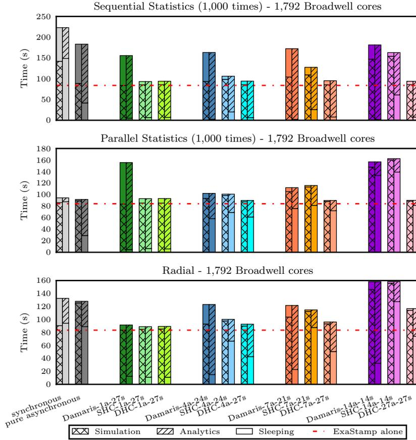
**Fig. 4.** Comparison of the different strategies on 1,792 Broadwell cores (64 MPI processes) for three analytics equivalent to or larger than the simulation timestep: sequential statistics performed 1,000 times (a), parallel statistics performed 1,000 times and radial.
