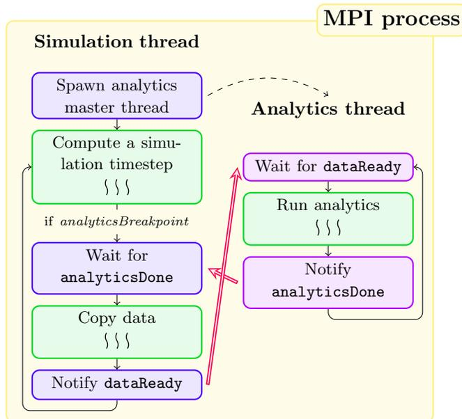
**Fig. 1.** Timeloops of the simulation (left) and analytics (right) master threads inside one MPI process. The green-framed blocks contain sequential regions (MPI communications for example) and parallel regions where simulation or analytics tasks are scheduled on the worker threads spawned by TBB inside the MPI process. The red arrows depict the synchronization between the master threads.
