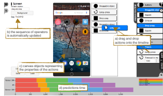
Figure 1: Example of StEM use: (a) the user drags and drops actions onto the timeline to construct the sequence of interaction of the current application screen; (b) the corresponding sequence of operators is automatically updated; (c) the user specifies the parameters of an action by manipulating its canvas representation (eg position, size, ...); (d) after querying the database, the prediction times are displayed as stacked bars (each colour represents an operator).
