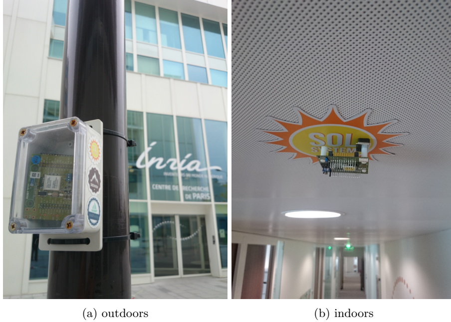
Figure 2: Devices deployed in the Inria-Paris offices for the Smart Building use case.
