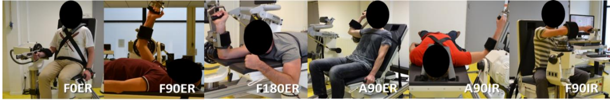
Figure 1. Natural and awkward shoulder configurations tested for elbow torque on dynamometer.
