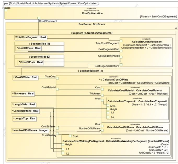
Fig.8. SysML PAR of the cost optimization function and related constraint blocks.
