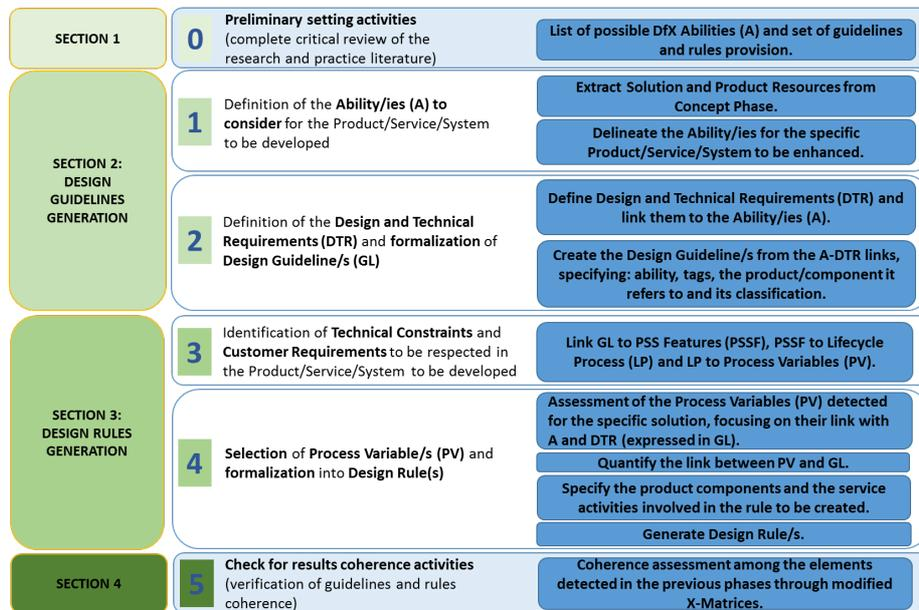
Fig. 1. The PSS design Guideline/Rule methodology (adapted by[9])
