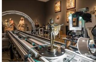
**Fig. 3.** CultLab3D Professional Scanner
